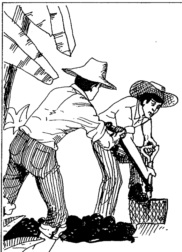
FIGURE 9.26 THE TWO-PERSON SHOVEL A simple, non-firing digging system for drains, gardens, and terraces.
